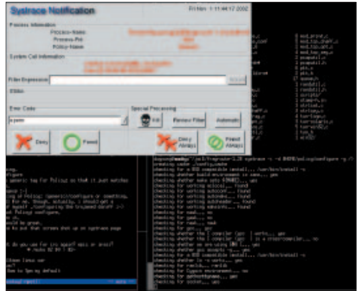
Figure 4: Systrace catches the configure script in a trojaned version of fragroute: The source package has been manipulated by malevolent hackers and attempts to open a TCP connection to port 6667 on IP 216.80.99.202
