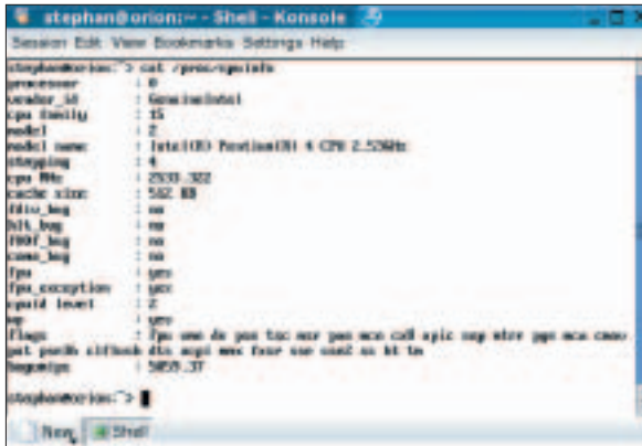
Figure 3: The cat /proc/cpuinfo command the processor characteristics supported by your kernel. The flags line indicates that this Linux version is aware of MMX, SSE, and SSE2 (Kernel 2.4.20)
