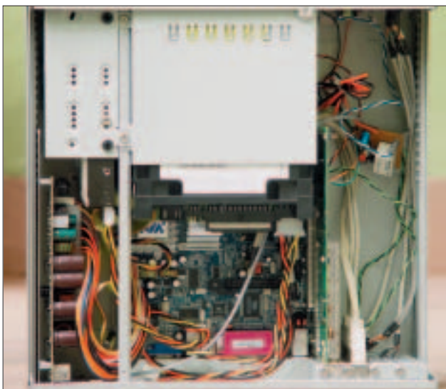
Figure 1: The case is compact, but provides ample space for a video recorder with a CD drive and one or two hard disks. As fanless operation is possible, the hard disk is the only source of noise, however, the operating temperature is about 40 degrees
