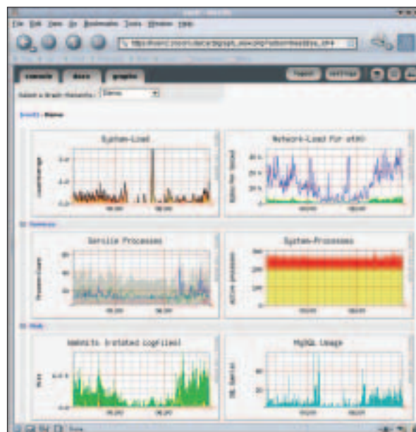
Figure 1: In the overview Cacti displays any graphs you have configured as thumbnails. Clicking a thumbnail opens the corresponding graph
