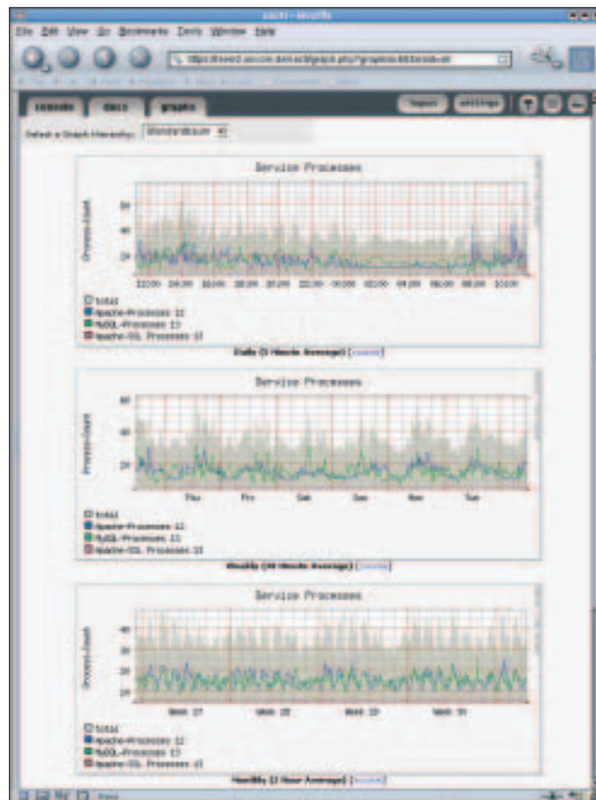
Figure 5: The detailed view displays four graphs with different sampling rates by default. This allows you to monitor current processes over an extended period of time
