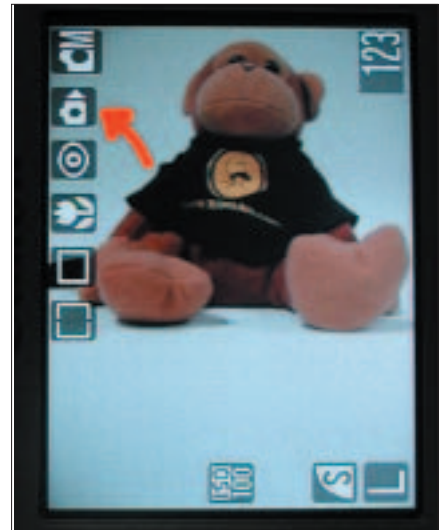
Figure 5: The Canon Digital IXUS 400 automatically recognizes whether the camera was held horizontally or vertically – as shown (marked with the arrow) by the orientation symbol on your screen – and stores all the photos in landscape format, while recording the correct orientation in the EXIF header
