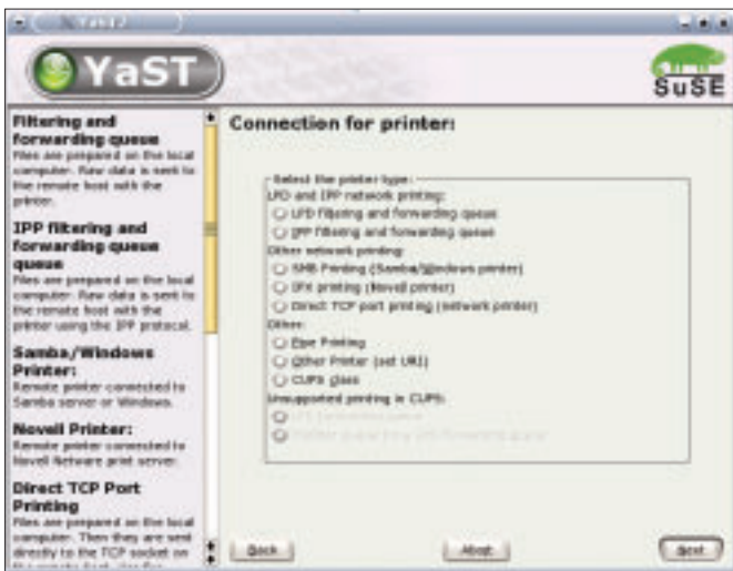
Figure 5a: Setting up remote printers on Suse Linux 8.2. First, tell YaST that you want to access a remote printer that uses IPP ...
