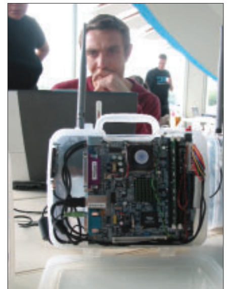
Figure 1: Portable wireless nodes. Mini ITX computers are concealed in the Rollergirls' cases.
