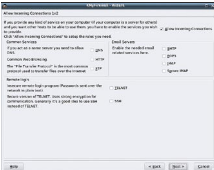
Figure 1: The wizard helps you set up KmyFirewall.
